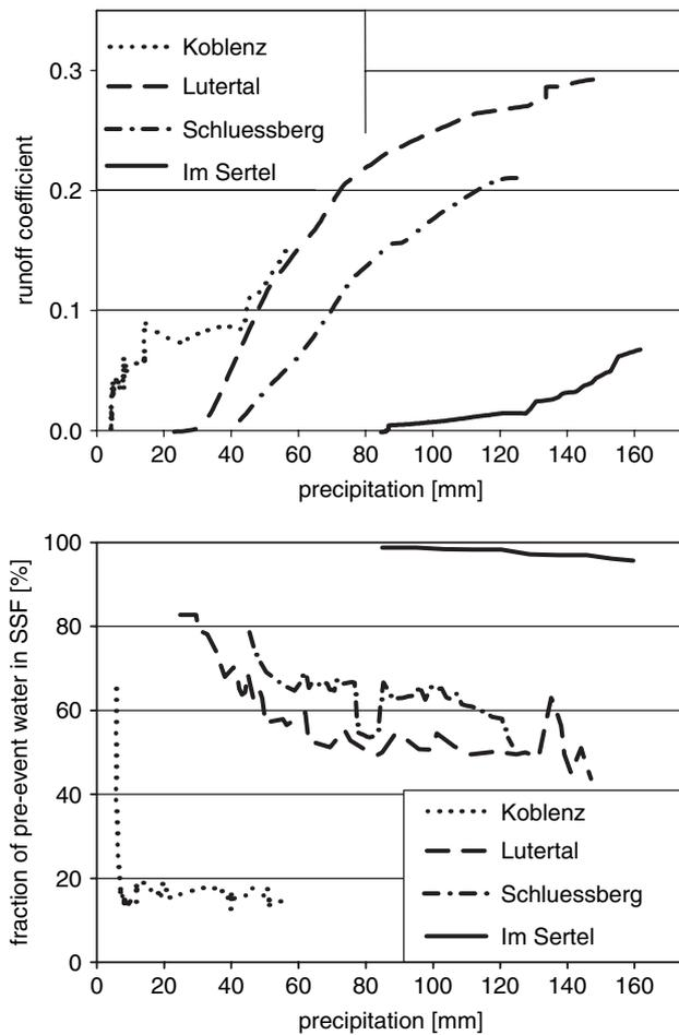
Figure 7. Intercomparison of differently responding hillslopes. Directly fed SSF starts quickly and contains little pre-event water (Koblenz). Indirectly fed SSF starts delayed and consists mainly of pre-event water (Im Sertel)
