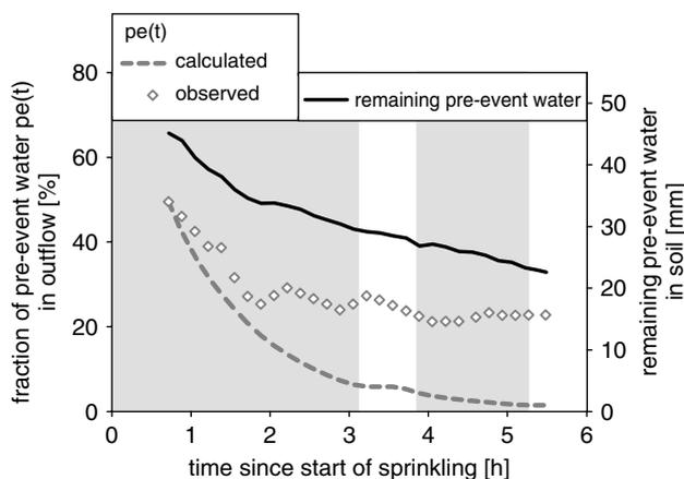
Figure 8. Comparison of observed pre-event water fractions  $pe(t)$  and calculated  $pe(t)$  assuming a complete mixing and 17 mm of movable pre-event water. The axis on the right-hand side refers to the amount of remaining pre-event water in the uppermost soil layer (solid black line)
